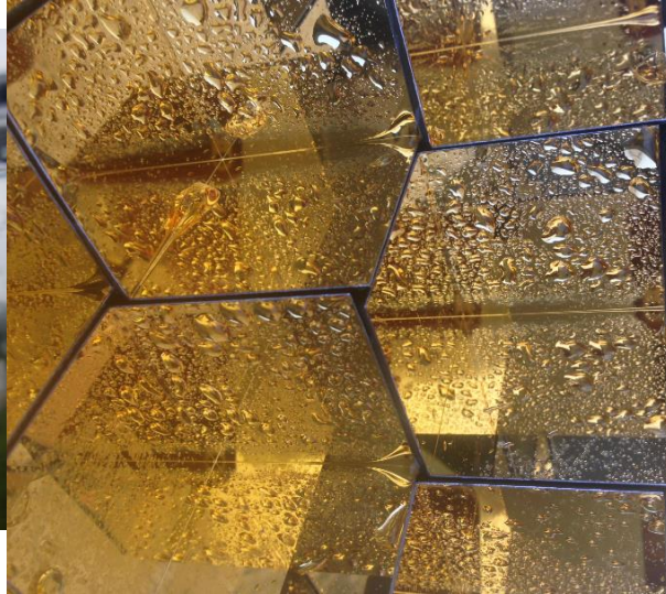
Water (rain/dew) on a retroreflector
