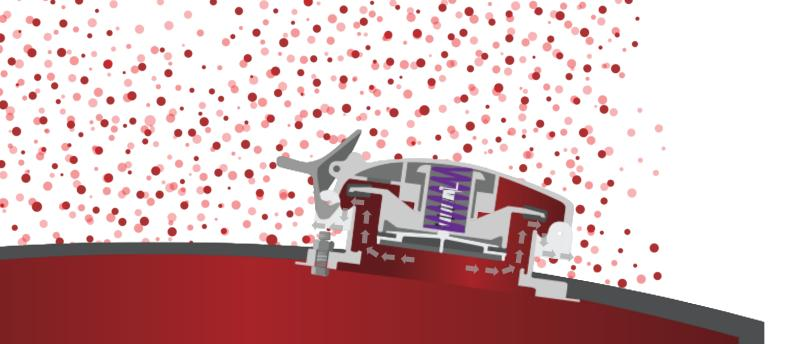
Tank systems are designed to open to atmosphere during over-pressure or vacuum conditions to protect structural integrity
