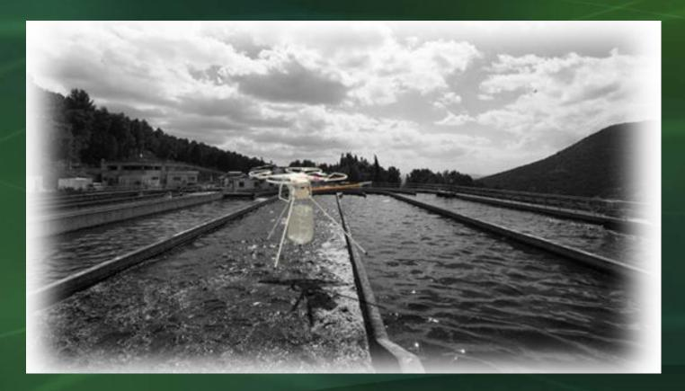
Drone used to Monitor air quality on wastewater system <a href="http://scentroid.com/scentroid-sampling-drone/">http://scentroid.com/scentroid-sampling-drone/</a>
